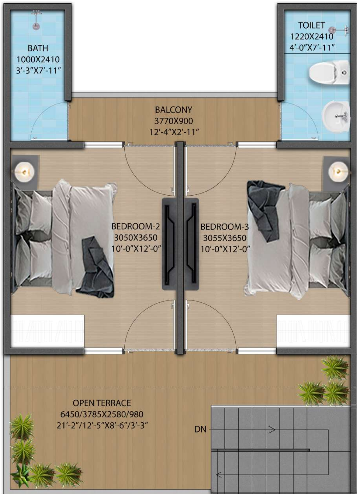
81 SQ.YD. VILLA FIRST FLOOR PLAN
